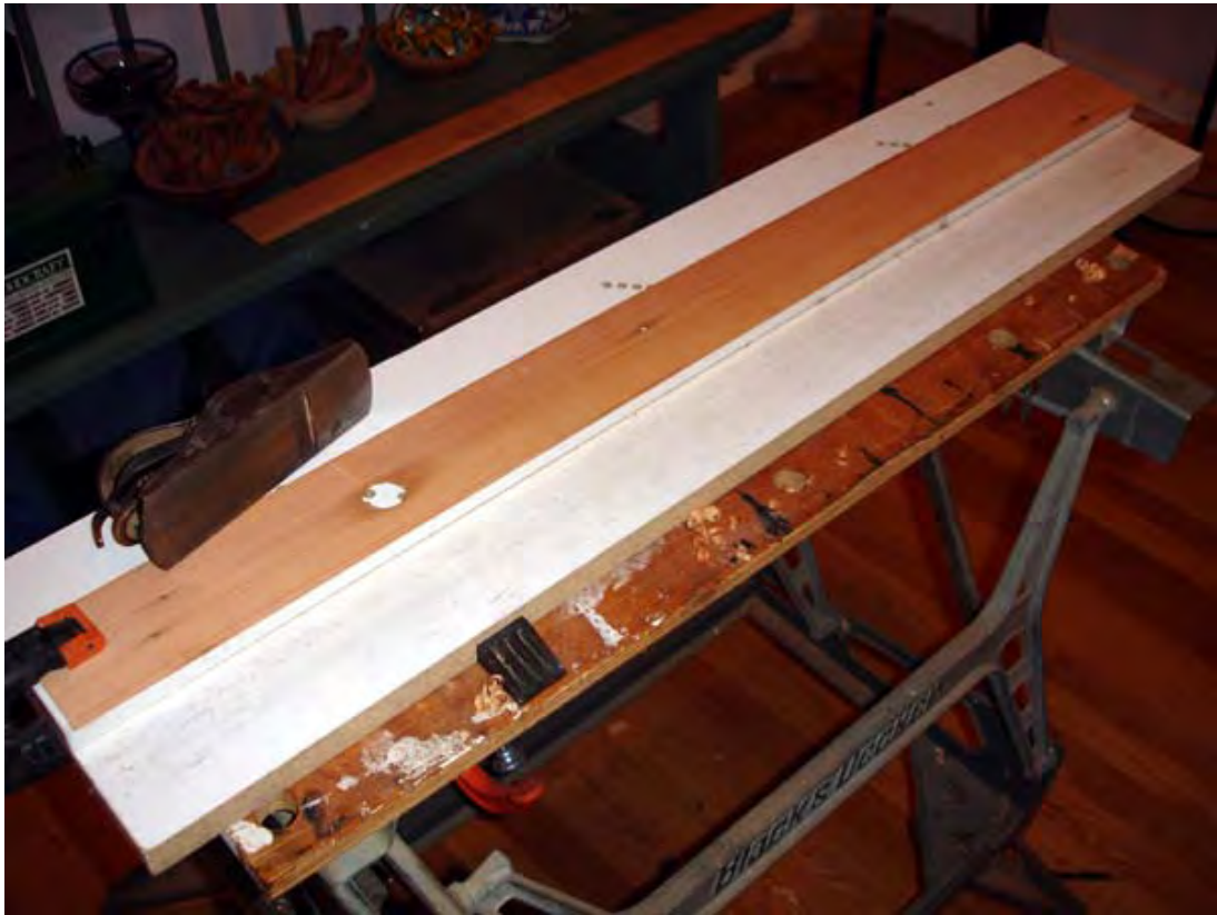
Here one of the sides of the instrument is planed and trued on its edges. It includes a 3/4" conduit hole and holes made by nails and insects.
