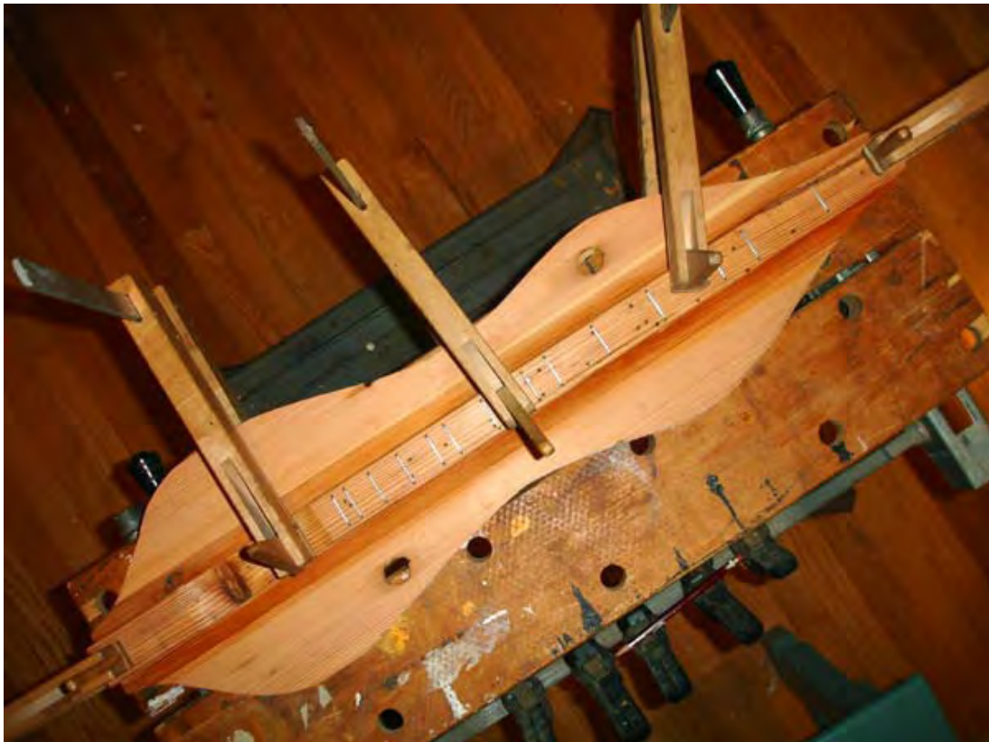
After the frets are in place the fretboard could be glued to the top. The old plaster lath nail holes make an interesting background pattern.
