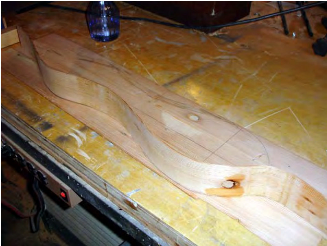
One of the sides is bent. The sides of this instrument are thicker than usual to counter the structural liabilities of the various defects. Usually my dulcimer sides are 2mm thick, these are twice that thickness.
