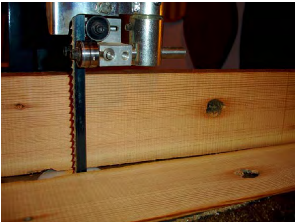
The piece with the most quartersawn cut is selected, planed and sliced into the side wood.
