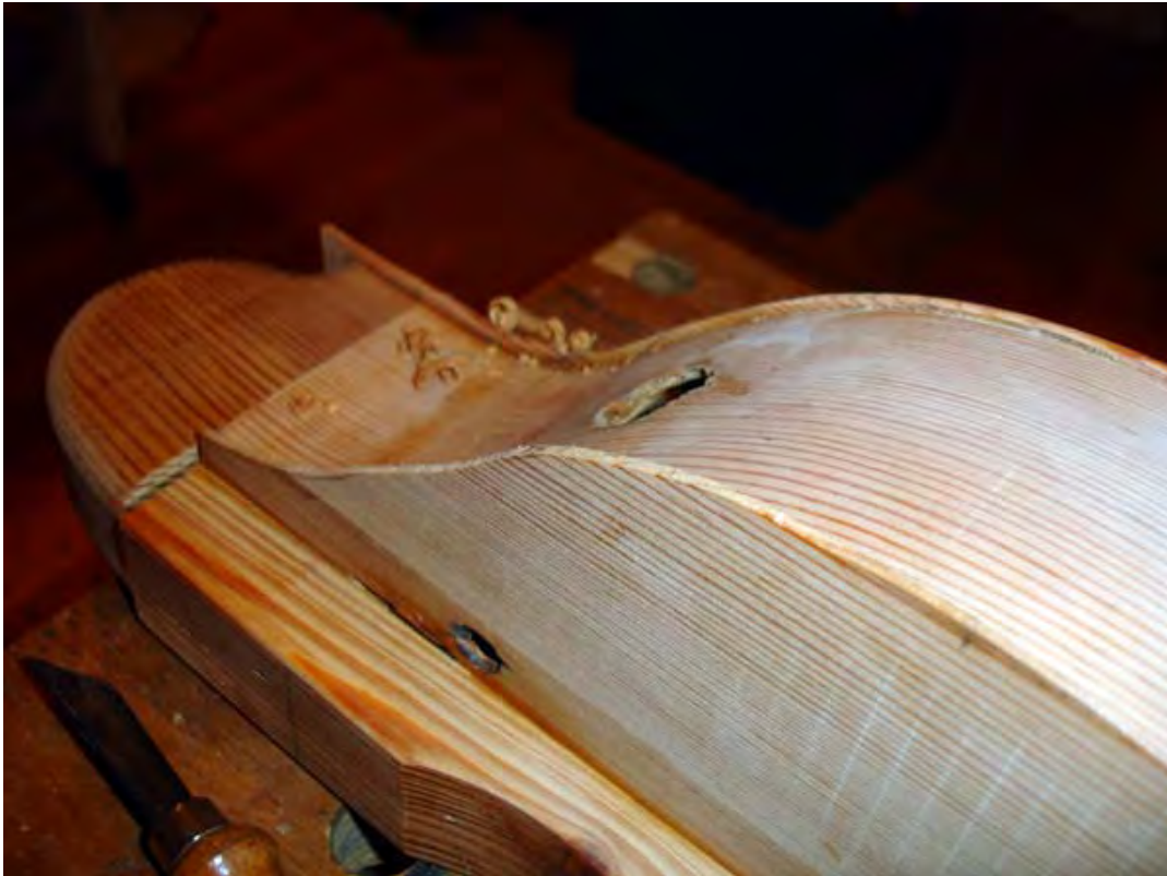
The top is attached and the edges are being trimmed. A hallmark detail of the earliest dulcimers is the presence of 'overlapping edges' as opposed to flush edges that are used on most modern instruments. This detail is reminiscent of the fiddle, which was probably the most familiar 'store bought' instrument to the rural makers.
